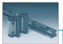
AccuMax\* Linear Roller Bearing System • Twice the load capacity of linear ball guide systems • Twice the rigidity of linear ball guide systems • Offers the Arcuate Advantage\* a patented design which includes cylindrical rollers on continuously crowned races
