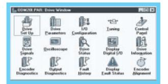
With just a click, the drive can be configured for a wide variety of operational modes (torque, velocity, position, step/dir, follower, etc.) Communications parameters may be set for single or multi-drop operation.
