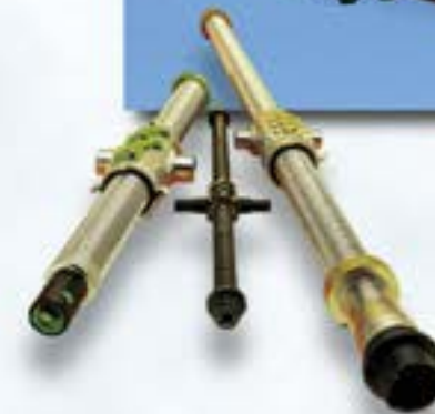
737 Wing Flap Ball Screws
