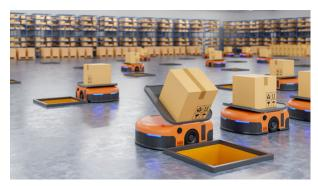
Long-life electric actuators have created a new, affordable solution for automated guided vehicles (AGVs), which can run all day and night and perform frequent linear motion tasks.
