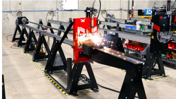
Thomson customized a motion control assembly that integrated a stepper-motor-driven lead screw into a previously ball-screw-driven linear slide.
