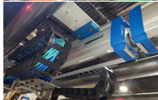
*The Movopart units attach to the system's stepper motors via Thomson RediMount™ motor mounting adapter kits, which enable seamless installation in only a few minutes.*
