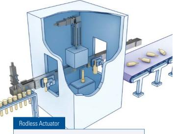
Here we illustrate how a Thomson rodless electric actuator can make the more commonly used hydraulic cylinder obsolete, providing better control, higher speed, simpler design, less energy consumption and a more environmentally friendly solution.
