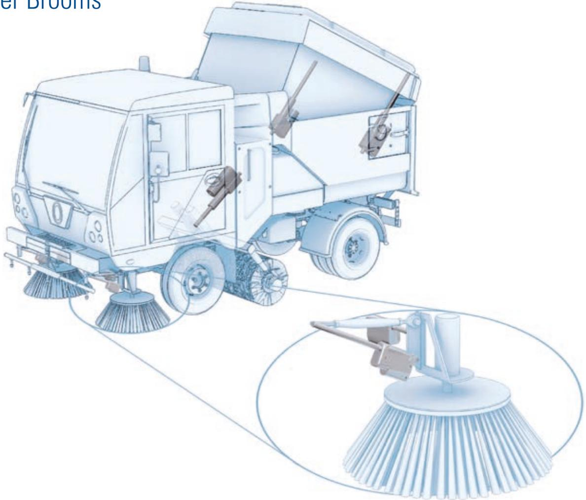
Actuators replace hydraulic and pneumatic cylinders for better controllability, smaller installations and eliminating the need of maintenance.
