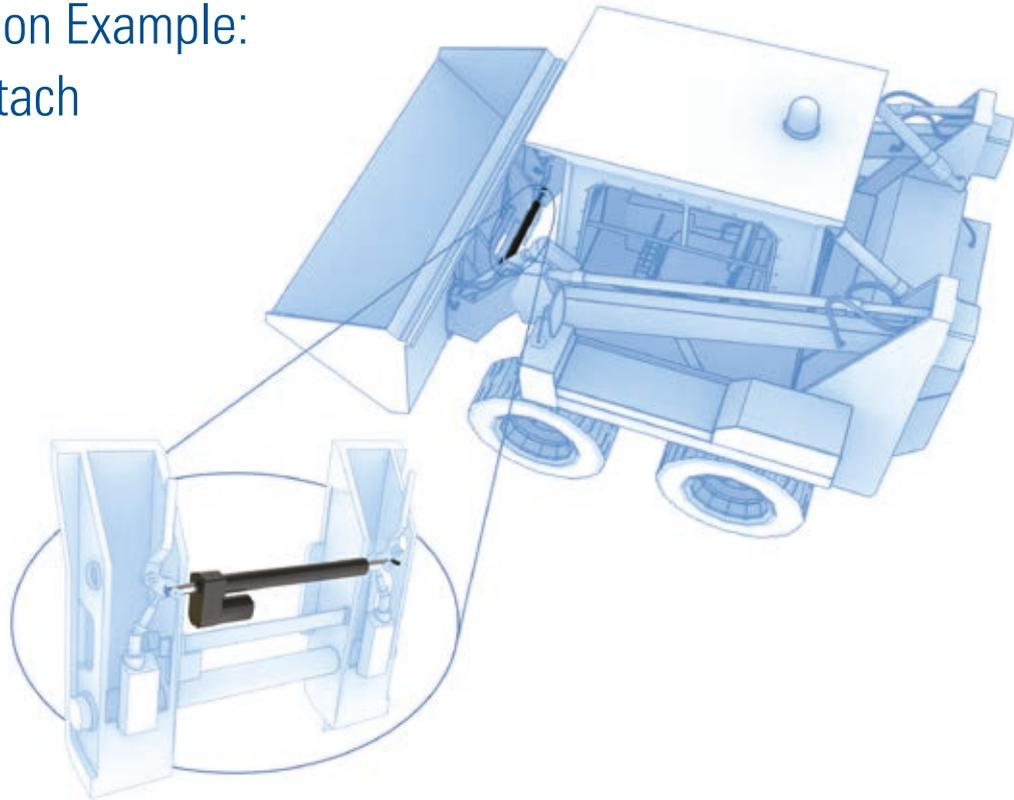
Quick-attach actuators allow the operator to change implements on the loader or skid steer without leaving the seat for improved productivity and safety.
