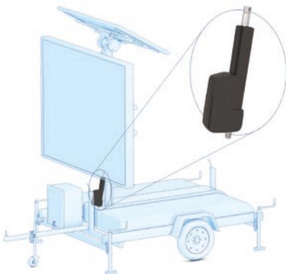
Long stroke, protection against harsh environments and high load rating makes linear actuators a great fit for this roadside construction sign.
