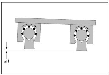
Since round rail linear bearings are free to rotate around their shafts, height mismatch does not result in binding.
