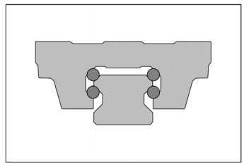
This cross section of a profile rail bearing illustrates how the balls are captured between the carriage and rail, both having races with close conformity to the balls.
