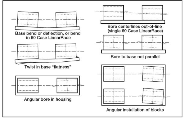
The self-aligning design of round rail ball bushing bearings allows them to be installed into imperfect systems. Normally four bearings installed in square pillow blocks are used to support a load and connected by a carriage plate.
