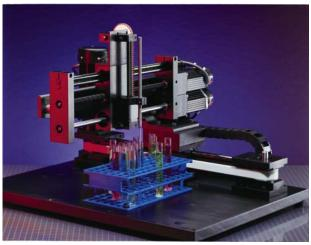
A fluid dispensing device that benefits from end supported round rail bearings which are captured in simple end plates, span a gap and offer smooth motion for this laboratory type application.
