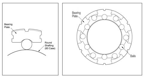
Cross section of a round ball bushing bearing showing how the balls ride between the bearing plate and round shaft and the manner in which the plates are arranged in a housing to contain the ball circuits.
