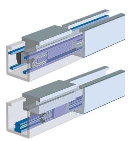
The sealing or protective covering for a linear unit includes no cover at all, bellows, shroud, or enclosed (ideal seal). Standard grease or clean room grease options are available for lubrication within the linear unit.
