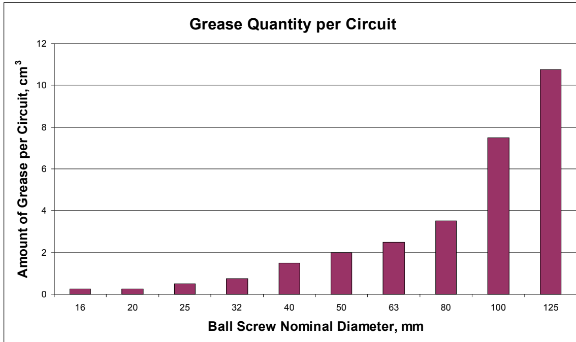
Figure 4 - Guide to grease quantity per circuit. To determine total volume required, you must multiply the volume determined from this figure by the number of circuits in the ball nut.
