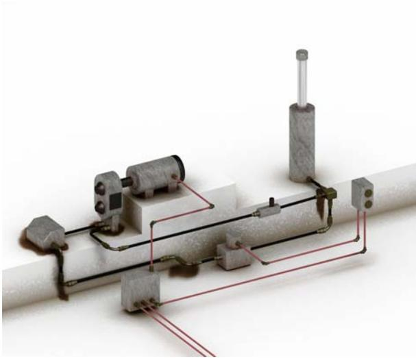
This single acting, uni-directional hydraulic cylinder system is one of the simplest hydraulic solutions available. It consists of eight parts that must be taken into consideration during the design process and installed by the OEM. For bi-directional operation, a more complex and costly bi-directional system would need to be installed.
