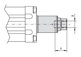
The inside thread option comes mounted from factory if this is stated in the ordering key at order. Possible types for the different unit sizes depend on the ball screw diameter of the unit, see "Ball screw diameter" in the table.
