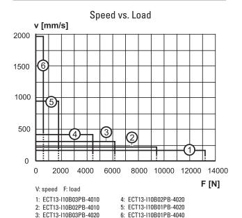
••••• = Overheating of the motor may occur if running at this speed continuously!
