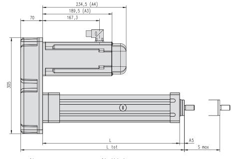
S max: maximum stroke (ordering stroke in mm) L: cover tube length L tot: retracted length
