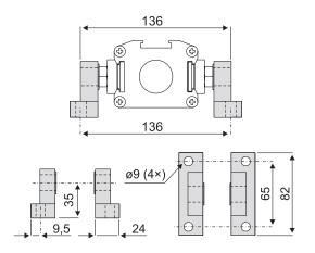
The trunnion option can be mounted on the unit from the factory if this is stated in the ordering key at order, or be ordered separately using the part number. When ordered separately, all necessary screws to attach the trunnions to the unit are included. The position along the profile can be adjusted freely by the customer. A trunnion bracket kit is available for T60, which is ordered separately.
