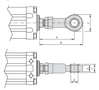
The spherical joint option can be mounted on the unit from the factory if this is stated in the ordering key at order, or can be ordered separately using the part number(s). When ordered separately, all necessary components to attach the spherical joints to the unit are included. Type M joints include a grease nipple. Note: When ordering a spherical joint separately, make sure that the extension tube end has an outside thread adapter to be able to mount it.
