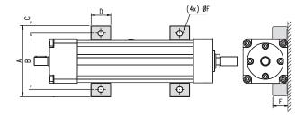
The movable mounting feet clamp accessory is only available for T60 units. This option can be mounted on the unit from the factory if stated in the ordering key at order, in which case you get four clamps, or they can be ordered as separate pieces using the part number. Normally you would need four clamps per unit. The clamps fit into the T-slot running along each side of the unit.
