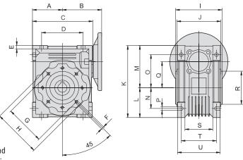
The worm gear is installed to the unit using a unit type and gear-size-specific adapter flange. No intermediate coupling is needed. The gear mounts directly to the motor and no coupling, bell house or adaptor flange is required. An optional rear clevis can be mounted to the gear by using a rear clevis adaptor flange. This can be ordered as a package either unmounted or mounted to the unit, or as separate items.
