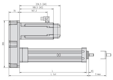
A1: power connector A2: resolver connector A3: without brake A4: with brake A5: ECT09-B53 • • • PB-25 = 15 mm, ECT09-B53 • • • PB-32 = 12 mm
