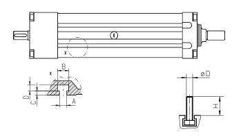
The T60, T90, T130, ECT90 and ECT130 models all have T-slots running along the entire profile. T60 has two T-slots (one on each side), while the other models have four (two on each side). Suitable T-slot bolts can be ordered using the part numbers in the table below.
