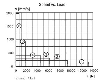
•••• = Overheating of the motor may occur if running at this speed continuously!
