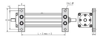
The fixed mounting feet are available for units type T90, ECT90, T130 and ECT 130 only. This option can be mounted on the unit from the factory if stated in the ordering key at order, or can be ordered separately using the part number. When ordered separately, all necessary screws to attach the feet are included. Note: The distance "G" can be different depending on the screw diameter of the unit.
