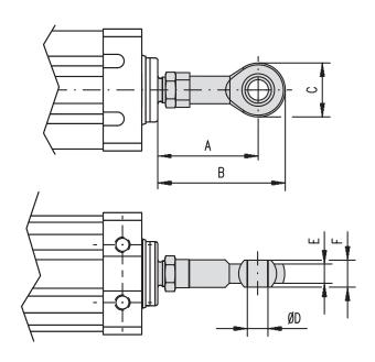
The spherical joint option can be mounted on the unit from the factory if this is stated in the ordering key at order, or can be ordered separately using the part numbers. When ordered separately, all necessary components to attach the spherical joints to the unit are included. Note: When ordering a spherical joint separately, make sure that the extension tube end has an outside thread adapter to be able to mount it.
