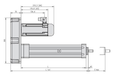
S max: maximum stroke (ordering stroke in mm) L: cover tube length
