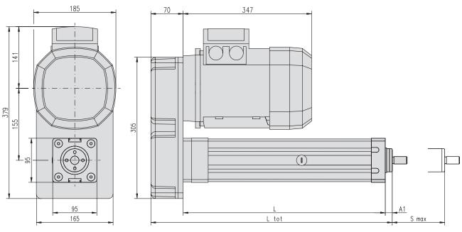
S max: maximum stroke (ordering stroke in mm) L: cover tube length L tot: retracted length
