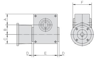
The worm gear includes a gear, bell house and matching coupling but no adaptor flange. The worm gear is ordered using the ordering keys on the right page. The adaptor flange is ordered separately using the part numbers below as there are different adaptor flanges depending on the type of unit being used.
