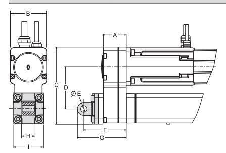
The rear clevis consists of a bracket and comes mounted from the factory if the ordering code states that the unit shall be equipped with one. It can also be ordered as a separate part (all necessary actuator attachment screws are included) using the part number.
