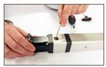
Tighten motor coupling screws and install sealing plug
