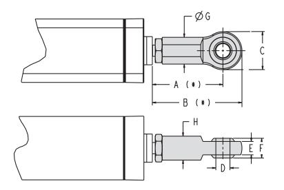
The spherical joint comes mounted from the factory if the ordering code states that the unit shall be equipped with one, but it can also be ordered as a separate part using the part number. To be able to mount a separate spherical joint, the extension tube must be equipped with a male threaded rod end.
