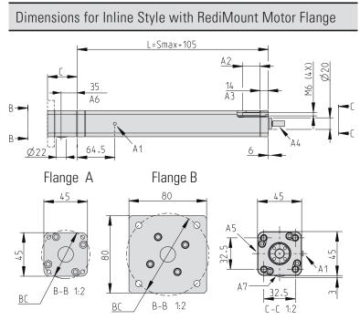
A1: grease port A2: M6 thread, max. depth 30 mm A3: no thread
