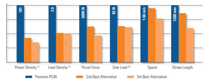
1) Power Density is defined as the maximum permissible force and speed compared to the frame size
