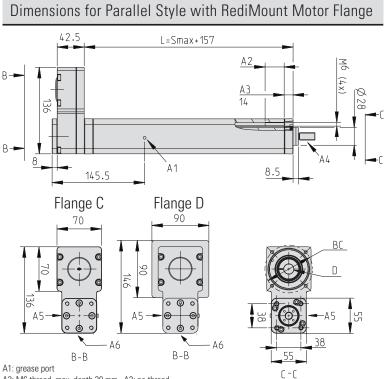
A2: M6 thread, max. depth 30 mm A3: no thread
