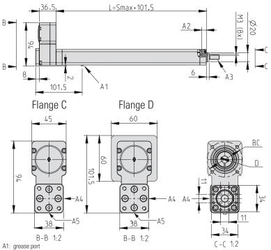
A2: M3 thread, max. depth 10 mm.
