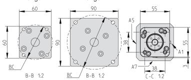
A1: grease port A2: M6 thread, max. depth 30 mm A3: no thread A4: male threaded rod end shown, see ordering key and accessories for information on all available ends. A5: side of cover tube for mounting of sensors. A6: distance to center of coupling tightening hole. A7: side of cover tube for coupling access hole and for mounting of foot mounts.
