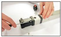
Tighten motor mounting screws
