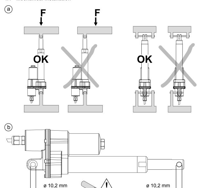
Always install actuator so that the force of the load acts in the center of the extension tube and the rear adapter and support the mounting pins at both ends (a). Only mount the actuator to the rear and front mounting adaptors using solid pins (b). The mounting pins must be parallel to each other both radially and axially and be supported in both ends.
