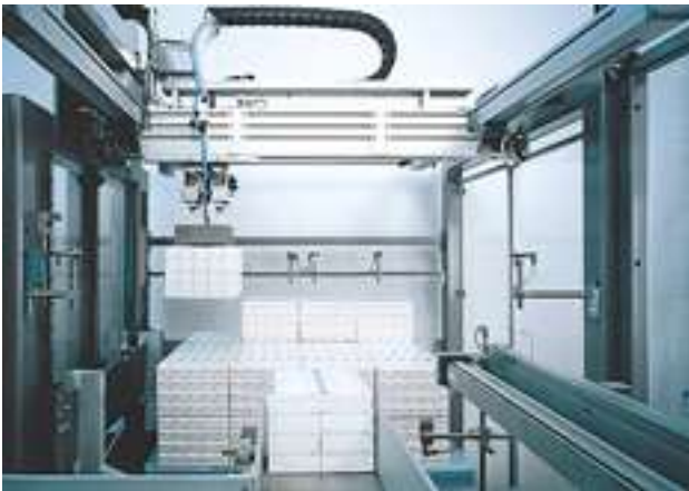
Robot palletizing application using linear motion system
