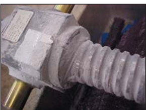
Milspec MIL-STD 810 sand/dust test
