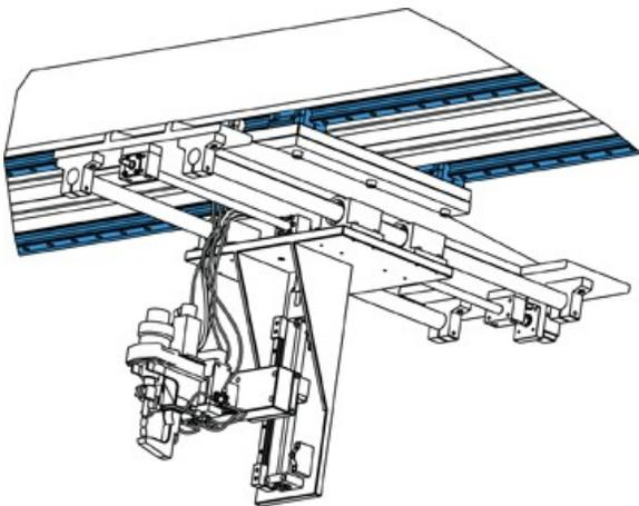
*Figure 5: 3-axis linear guide application*
