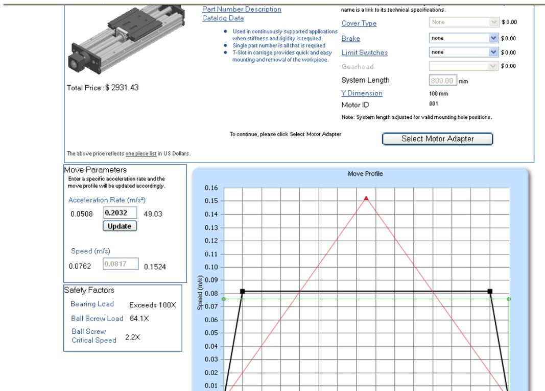
Figure 6: Application calculates minimum acceleration move profile (green), recommended move profile (black) and maximum acceleration move profile (red). Screen shot from Linear MOTIONEERING ([www.linearmotioneering.com](http://www.linearmotioneering.com)) web-based sizing and selection tool.
