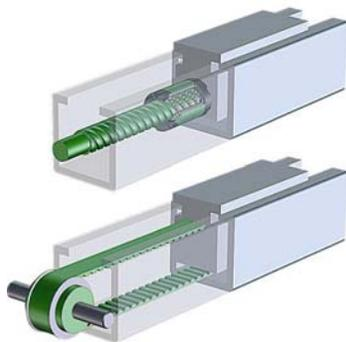
Figure 3: Ball screw drive (top) and belt drive (bottom)
